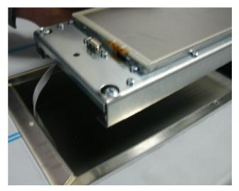
2 – Insert the connector and house the screen in the door.
