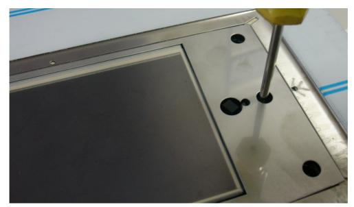
5 – Fix the screen in the final position with the 2 screws. Check that the alignment does not change. If required loosen the 2 central screws and adjust the position again with the screws in the corners.
