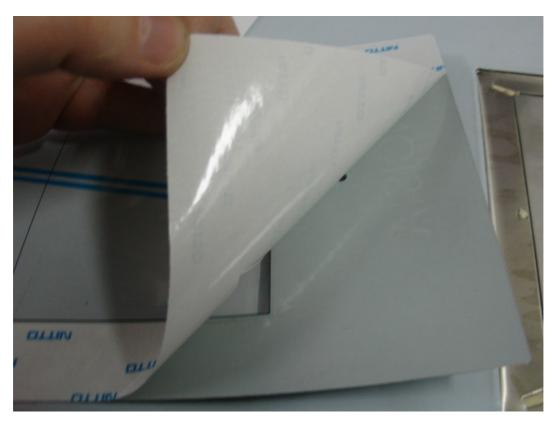
8 – Remove the protection layer on the adhesive side of the cover and attach it starting from the top downwards.
