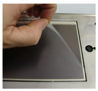
7 – Remove the protection film from the polycarbonate cover and from the touch screen.
