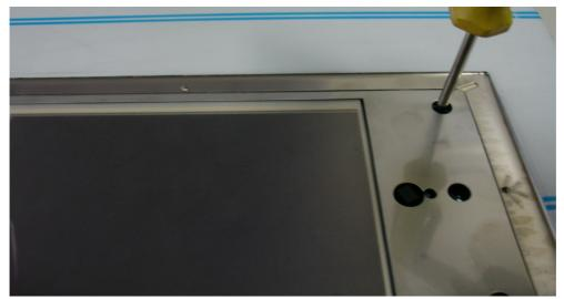
4 – By adjusting the 4 screws in the corners, line up the surface of the screen with the edges of the cover plate.
