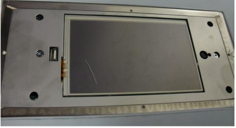
3 – Fix the screen with the long screws and place the cover plate. (stop the plate with scotch tape during this operation).
